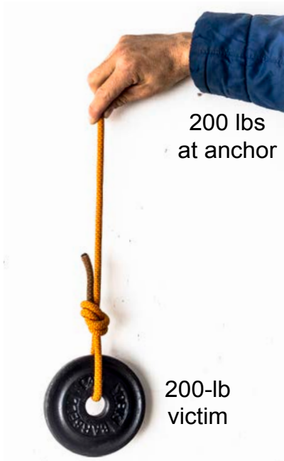
1:1 direct haul with no mechanical advantage.
