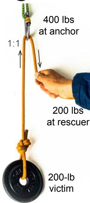
1:1 redirect with no mechanical advantage, but added friction from the carabiner.
