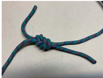
Flemish bend. For joining ends together for prusik loops and cordelette. 4- to 6-inch tails.
