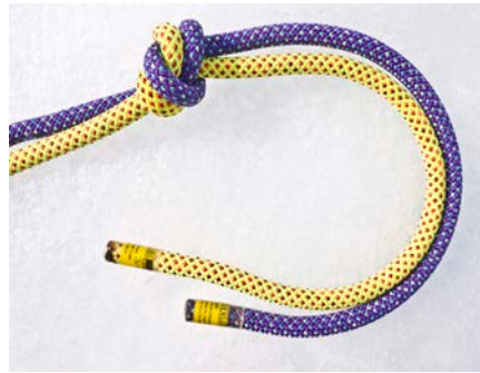
Flat overhand. For joining ropes for rappel. Dress and stressed with 18-inch tail.
