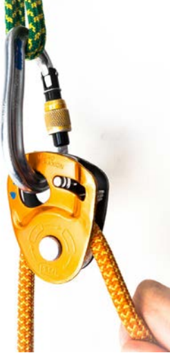
The 53-gram Petzl Nano Traxion is both a 91% efficient pulley and a cam for progress capture.
