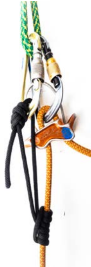
Prusik for progress capture using a belay device (e.g., BD ATC) to mind the prusik so it doesn't flip back through the master carabiner.
